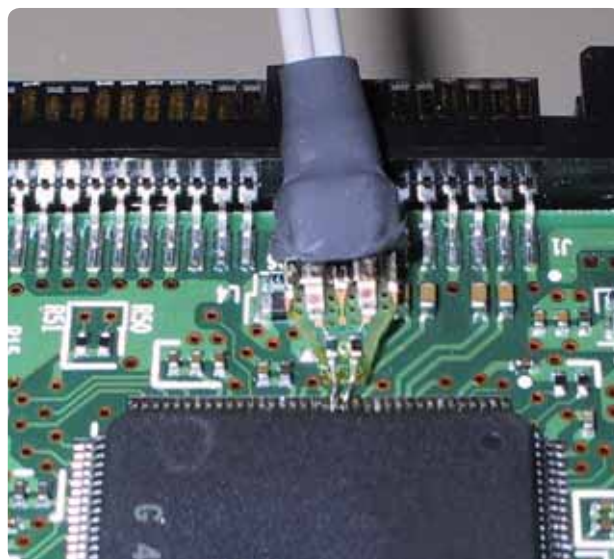
Figure 1. Differential active probe with 13-GHz bandwidth, connected to the TX package pins on a high-speed serial link.
