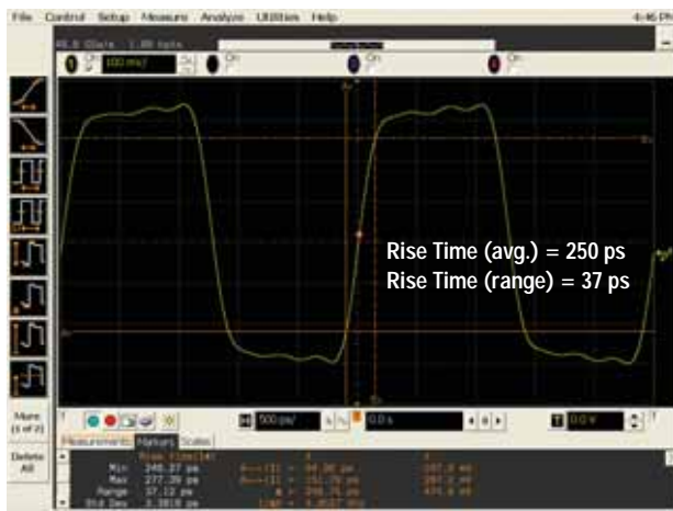
Figure 5a. 400-MHz clock captured on an Agilent Infiniium DSO80304B 3-GHz oscilloscope sampling at 40 GSa/s.
