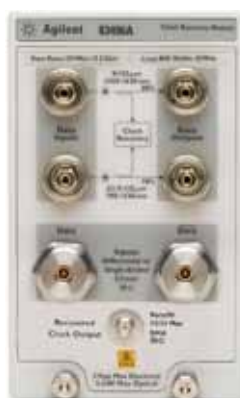
Figure 3. A key circuit in Agilent's 83496A multi-rate optical/electrical clock recovery module was designed in the InP HBT process. This is the industry's first clock recovery module with the necessary sensitivity and accuracy for high-speed waveform analysis at any data rate.
