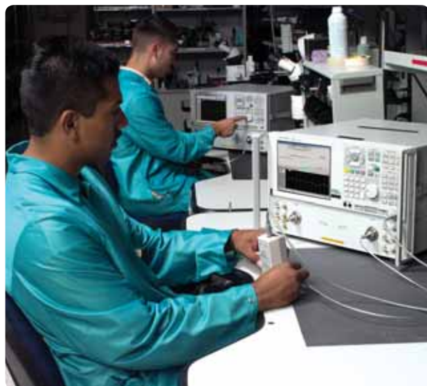
Figure 2. The Agilent N5230A 50 GHz precision network analyzer, which contains the InP HBT technology, enables microwave engineers to characterize components faster and increase production throughput while enhancing accuracy.
