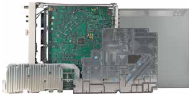
Figure 8. The discrete assemblies that make up the MXG signal generator.
