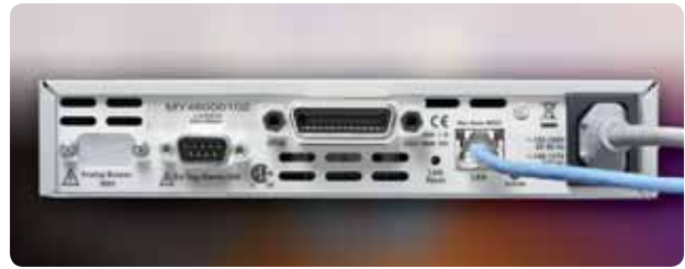
Figure 2. A modular LXI instrument uses the RJ-45 LAN connector (blue wire) to communicate with a PC controller through an existing LAN infrastructure.
